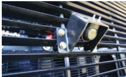
The WAVS camera by Caterpillar offers two camera view options: a panoramic 115 degree wide angle and 78 degree narrow angle.
