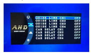
**GUIDE LINE CH1-4:** Allows user to turn ON/OFF guides. Guidelines appear only during triggered events. **CAR DELAY CH1-4:** Allows user to set duration of triggered camera on individual cameras.
