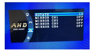
**ROTATE:** Allows user to rotate the whole image for all
