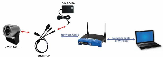
NOTE: Depending upon how the InnoPro camera is hooked up, camera can take up to 90 seconds to fully boot.
